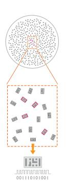
One of the image frames on the bottom of a 96-well microwell following target reaction, a mixture of BMBs can be simultaneously decoded and fluorescence (e.g. red) detected with proven optical technology.
